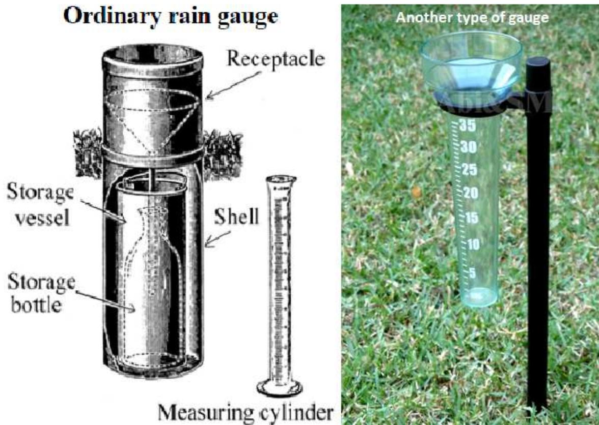
**Figure 3.1: Images of different types of rain gauges available for rainfall measurements.**
