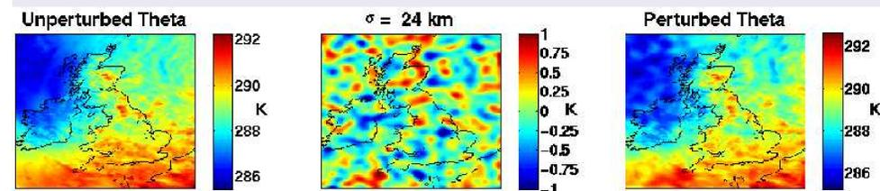
Figure 1. Example structure of perturbation field (scale length 24 km, amplitude 1 K) and effect of applying it.
