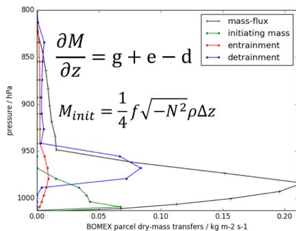
Fig. 1 Example of initiating mass flux profile for a BOMEX sounding.
