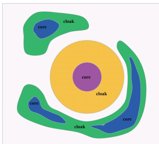
Fig. 2. The schematic diagram of our core-cloak representation of convection. Both downdrafts and updrafts are represented as a combination of core (strong draft) at centre and cloak (weak draft) around the centre.
