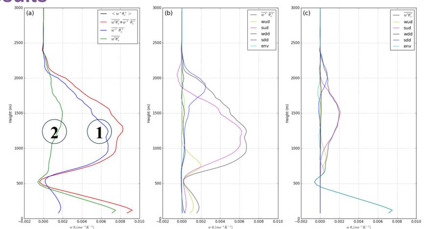
Fig. 3. Vertical profile of time- (last 1 h) and domain-averaged buoyancy flux and its different components in BOMEX simulation: (a). Total buoyancy flux (red solid lines), mass-flux contribution (blue line) and sub-plume variability (green line); (b). Mass-flux contribution (grey line) of total buoyancy flux and its components from different types of drafts; (c). Contribution from sub-plume variability (grey line) to the total buoyancy flux and its components from different types of drafts.
