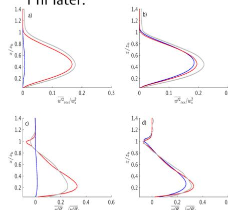
Figure 3. Normalized profiles of the resolved (a,b)  $w$  variance and (c,d) turbulent heat flux in the 400m simulation with PGB (blue) and DNB (red). (a,c) at 1140 and (b,d) at 1240. The coarse-grained LES profiles are in grey.
