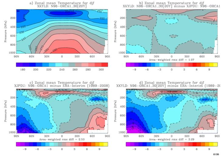
Figure 24: Zonal mean temperature (DJF) in the two model runs N96-ORCA1 (30 min) and N96-ORCA1 (20 min) as well as in observations (ERA40). Shown are averages over years 31 to 50 of the model runs.
