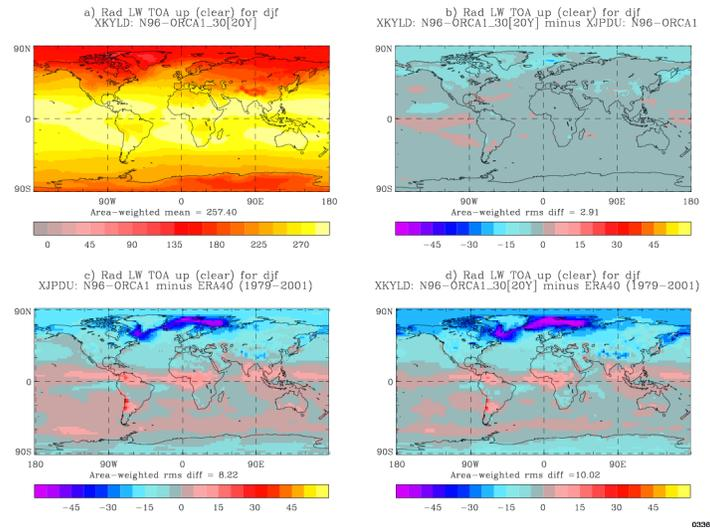
Figure 25: Clear sky outgoing longwave radiation (DJF) in the two model runs N96-ORCA1 (30 min) and N96-ORCA1 (20 min) as well as in observations (ERA40). Shown are averages over years 31 to 50 of the model runs.
